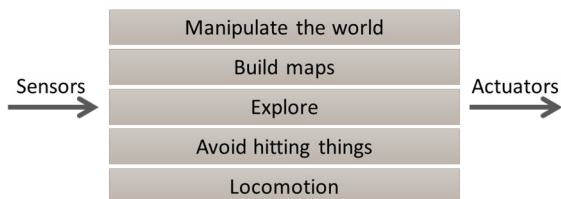
Figure 6. Layered control system according to Brooks [19]
