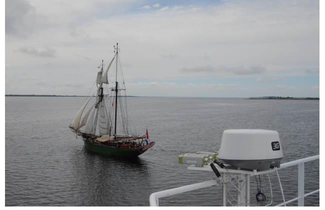
Fig. 4. Southern Funen archipelago. Sensor platform mounted beyond wheelhouse / ship's bridge.
